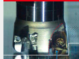
Cutting chips which were discharged well
